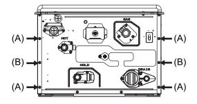
3 Insert the Pipe Cover to the clearance gap of (B) Screws. And re-secure above 6 screws.
