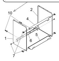
When fixing to the wall, this part can be slid 0.4" (10mm) to the rear by loosening the tapping screw.
